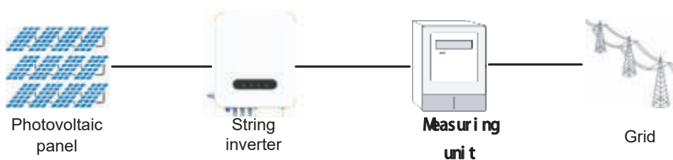
Figure 2-6 Application diagram of the string inverter network
